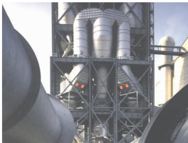
VSR BLASTER® air cannons in a cement plant (Foto: Krupp Polysius)
