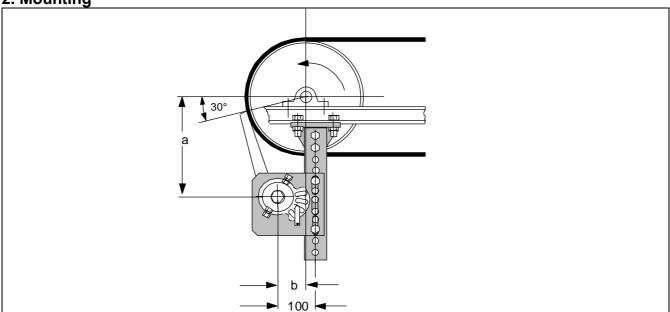
a) Take measure a - b to determine the centre of the axle in accordance with the drum diameter out of table (page 4).
