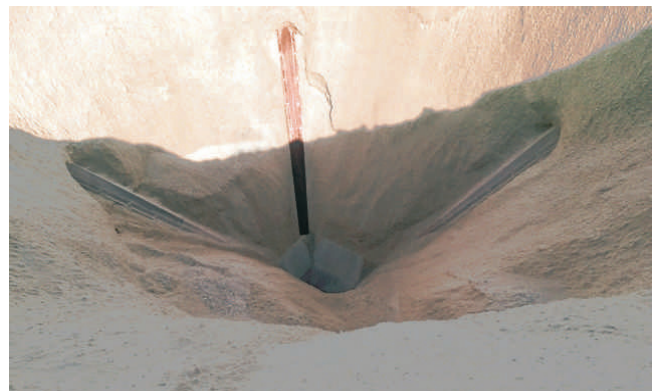
Isobaric sword nozzles remove and avoid discharge troubles. The stockpile capacity is increased.
