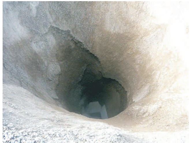
Without sword nozzles: Funnel and bridging formation, small active stockpile volume
