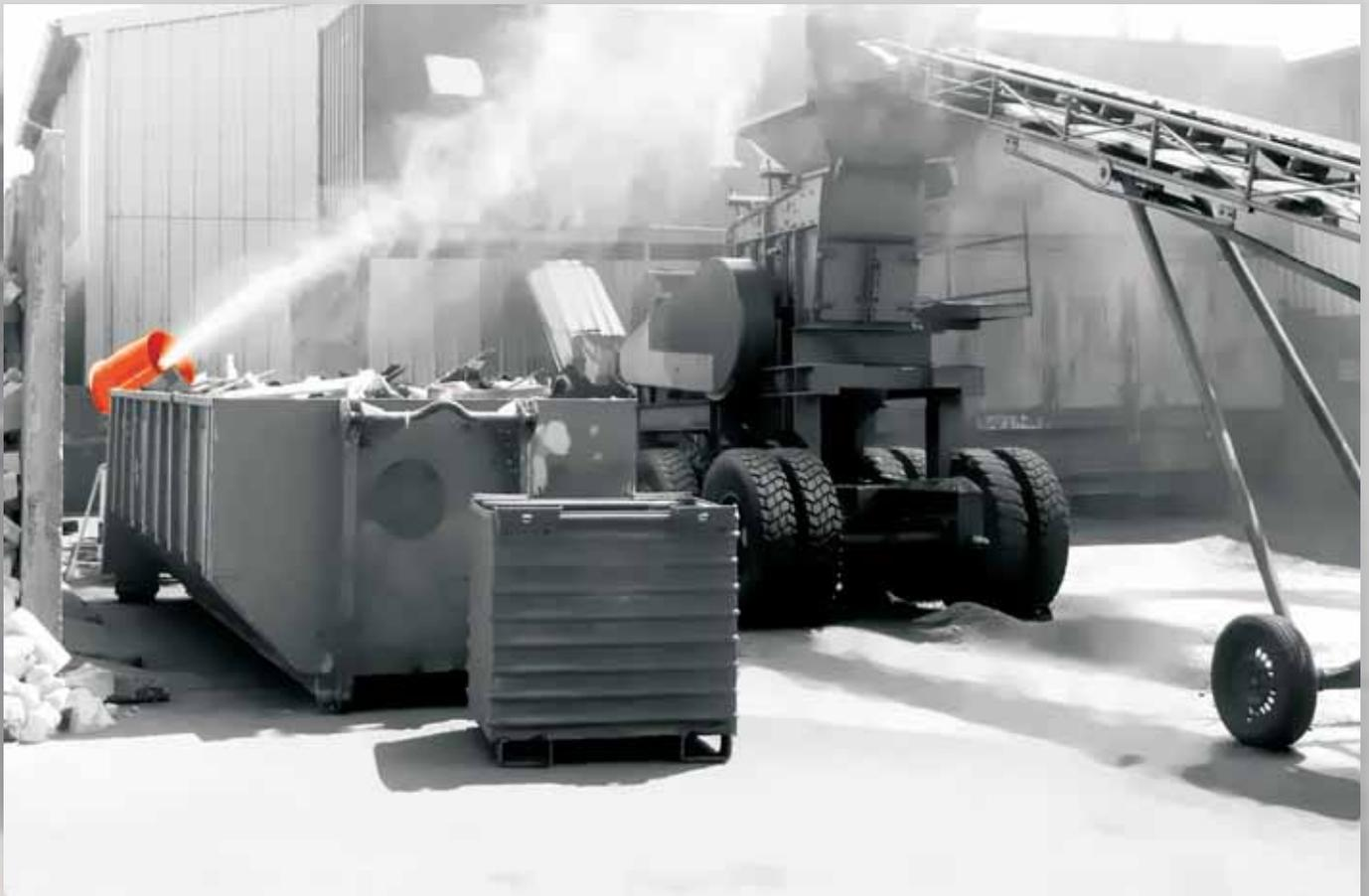
With a working pressure of 16 bar, the DUSTEX® Fog Blower creates a fine water fog with the applied nozzles that binds the dust particles directly at the source and reduces visibly the dust emissions.
